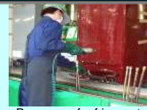
Recovery of refrigerant fluorocarbon from fridge
